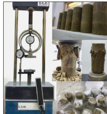
Fig. 1 Preparation and testing of UCS samples with additives.
