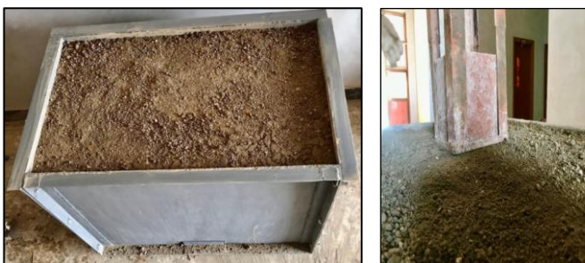
Fig. 4 Sample preparation for normal soil and treated soil.
