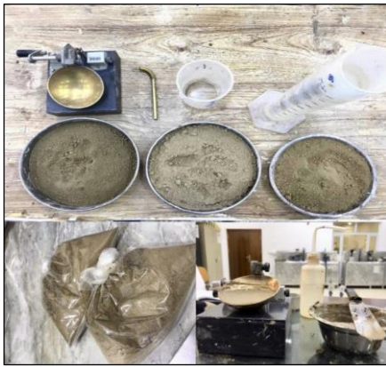
Fig. 2 Soil samples improved with chemical additives.
