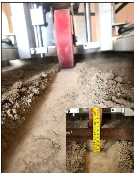
Fig. 17 The rutting occurred of the test samples.
